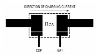
Figure 4 Kelvin Sensing of Charge Current
