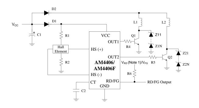
Note1: V<sub>RD</sub> should be equal or smaller than V<sub>CC</sub>
