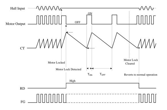
Note 5: Automatic restart is performed in the following manner. A motor lock condition is detected when the Hall signal stops switching. The output is ON when CT pin is being charged. C2 is the external capacitor of the CT pin. Output ON time and OFF time are determined by the capacitance of C2.
