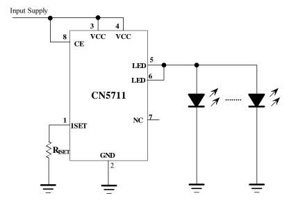
Figure 3 CN5711 drives LEDs in Parallel
