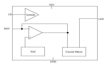
Figure 2 Functional Block Diagram
