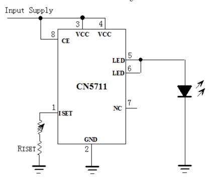
Figure 5 A Potentiometer to Dim the LED
