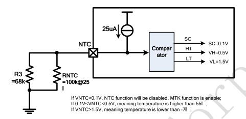
IP2163 integrated NTC temperature sensitive resistor detect function, and support abnormal temperature indication on FA pin. NTC and FA are multiplexed with CSN and CSP function on pin 1 and pin 2, only one function is enabled at the same time.
