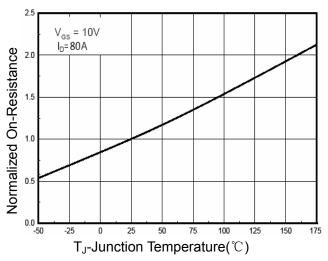
Figure 4 Rdson-JunctionTemperature
