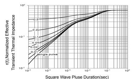
**Figure 11 Normalized Maximum Transient Thermal Impedance**
