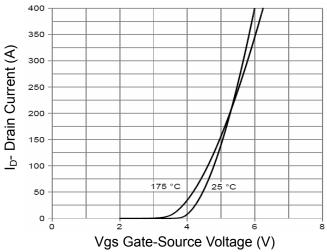
**Figure 2 Transfer Characteristics**
