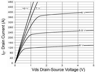
**Figure 1 Output Characteristics**
