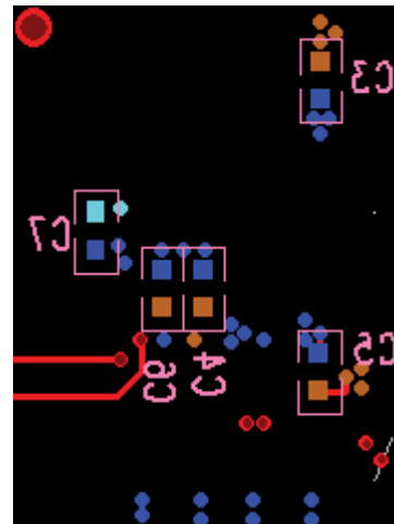
Figure 63. Bottom Layer Decoupling
