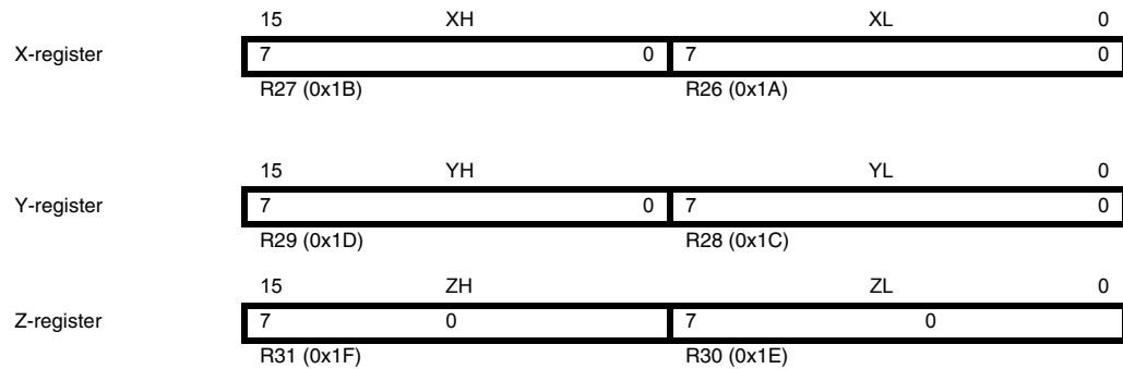
Figure 6-3. The X-, Y-, and Z-registers
