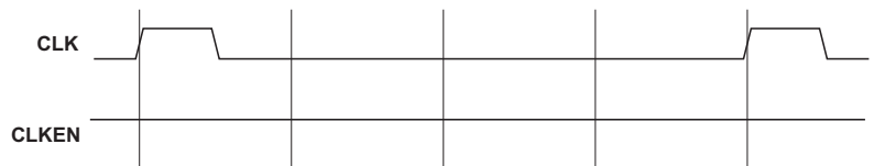
Figure 5-2 Stopping CLK for power saving
