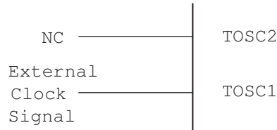
Figure 14-15. Timer/Counter2 External Clock Connections
