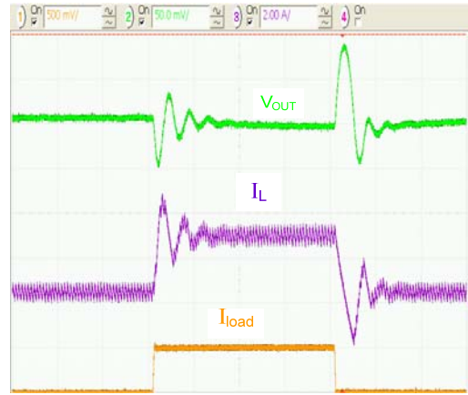
Figure 14. 500 mA to 3 A to 500 mA, 5 \mu\text{s}/\text{div} .
