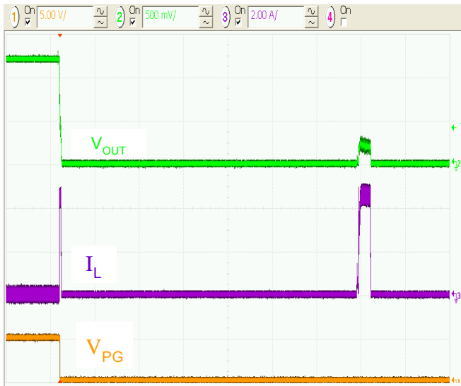
Figure 23. V OUT to GND Short Circuit, 200 \mu\text{s}/\text{div} .
