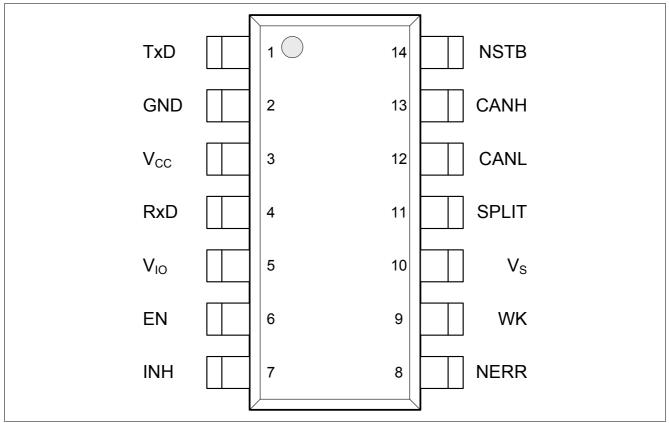
Figure 2 Pin Configuration
