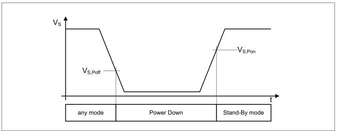
Figure 13 Under-Voltage on  $V_{\rm S}$
