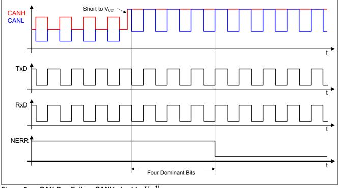
Figure 9 CAN Bus Failure CANH short to  $V_{cc}^{1}$
