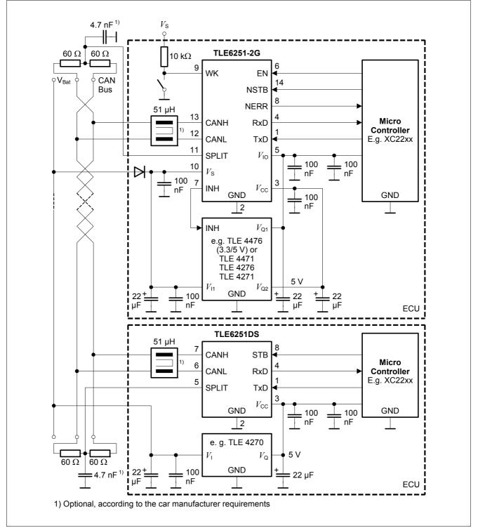
Figure 16 Application Circuit Example
