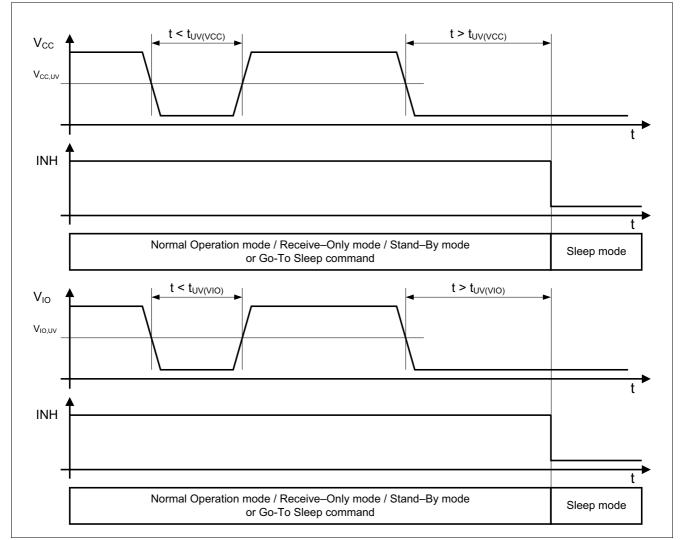
Figure 12 Under-Voltage on  $V_{IO}$  or  $V_{CC}$
