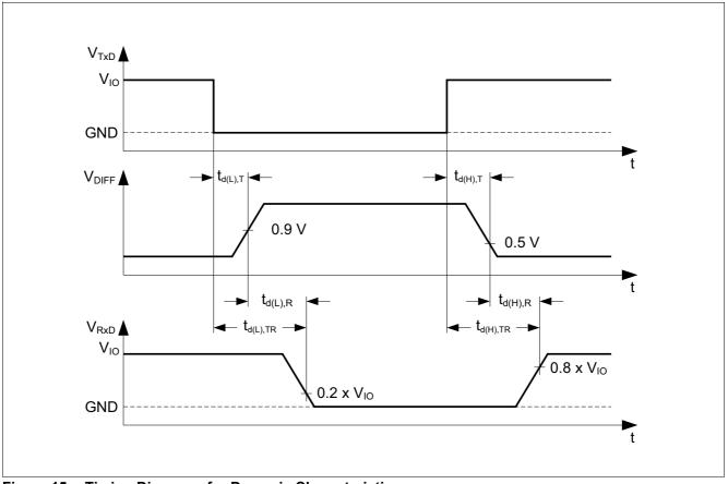
Figure 15 Timing Diagrams for Dynamic Characteristics
