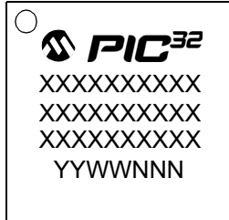
64-Lead QFN (9x9x0.9 mm)
