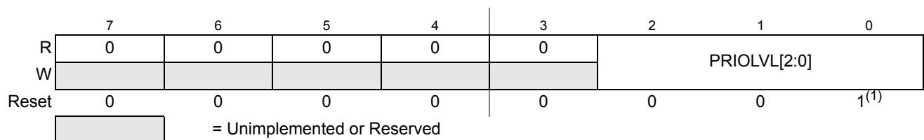
Figure 4-6. Interrupt Request Configuration Data Register 1 (INT_CFDATA1)
