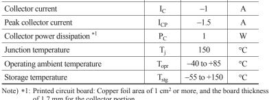
of 1.7 mm for the collector portion Absolute maximum rating without heat sink for P<sub>C</sub> is 0.5 W
